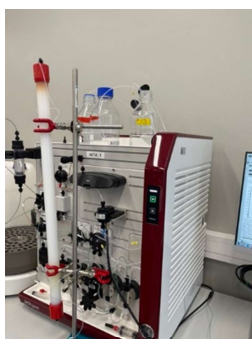
Figure 2.2. Size-exclusion chromatography (SEC) performed with a Sephacryl S-100 HR column using the Äkta
